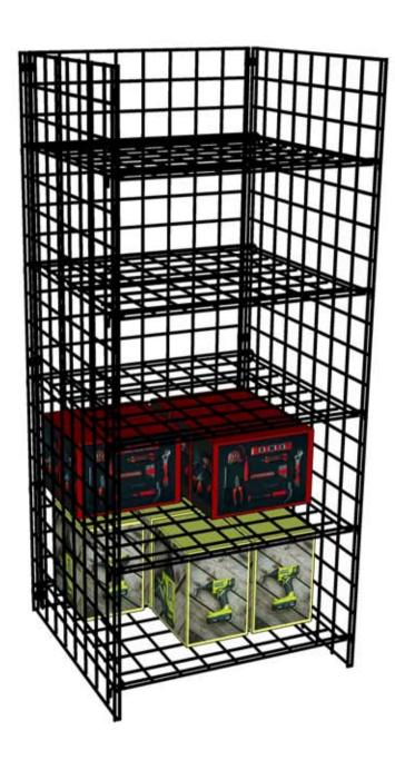
Step 1: Use connectors to connect edges of grid panels, using four connectors per edge. This may be done with grid panels upright or on floor. Use the two vertical bars that make up grid edge, connect to the inside bars.
